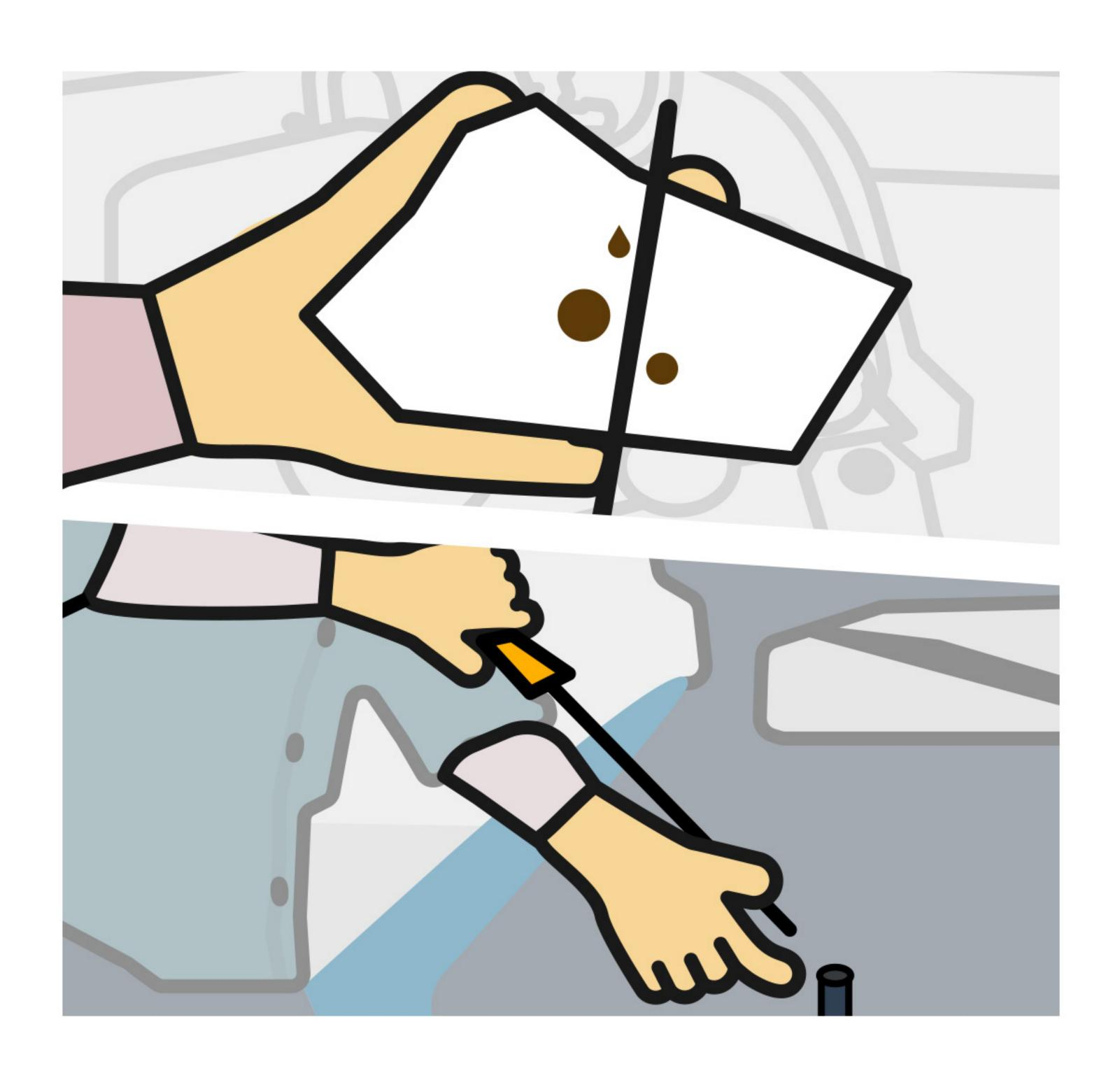
Remove dipstick to check oil level. Fill as needed.
