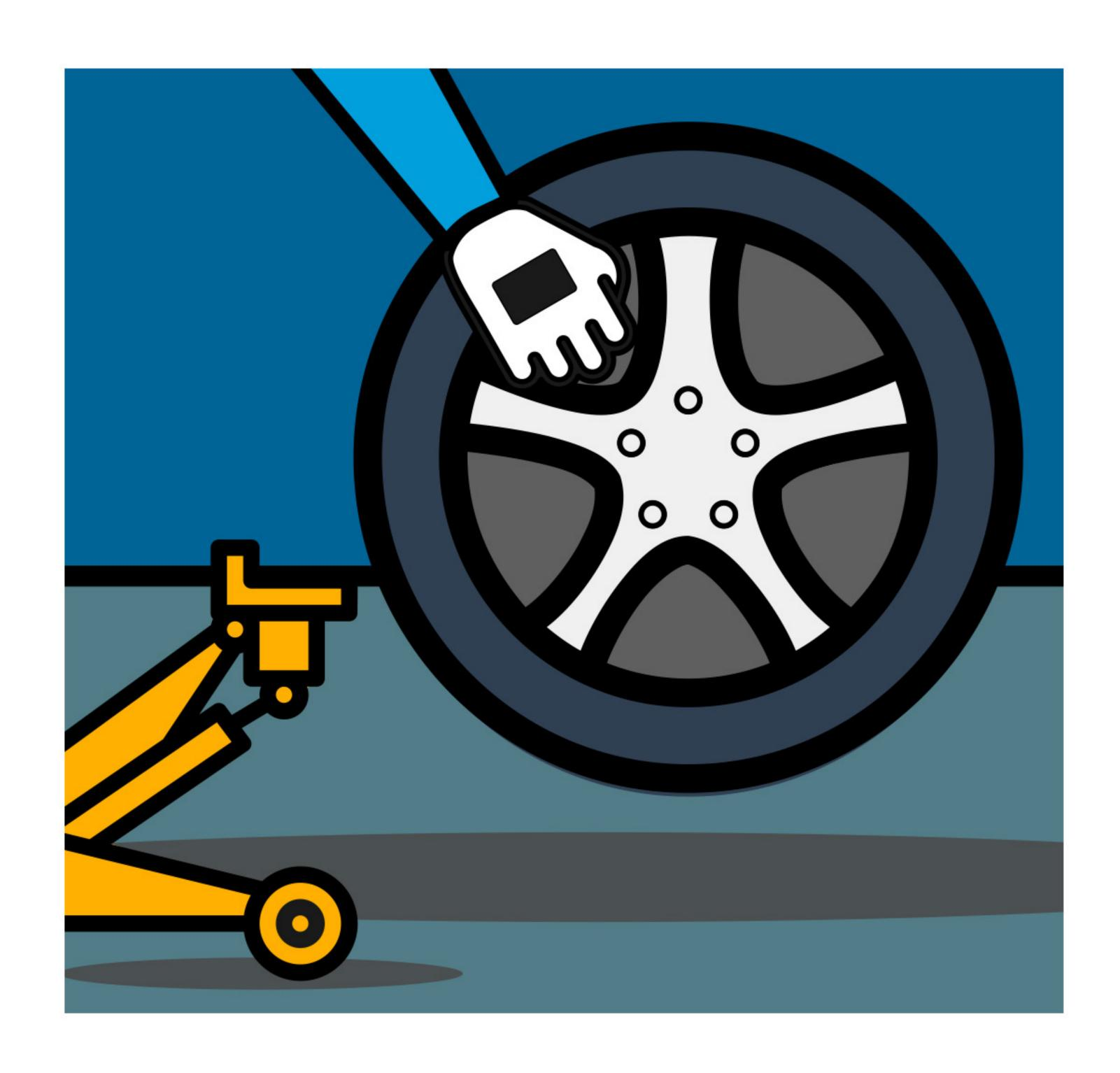
Replace lug nuts. Tighten by hand.
