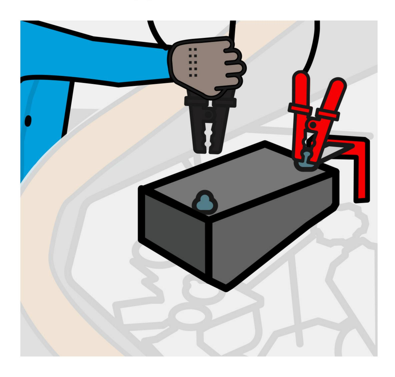
Remove red clamp from positive terminal of support car.
