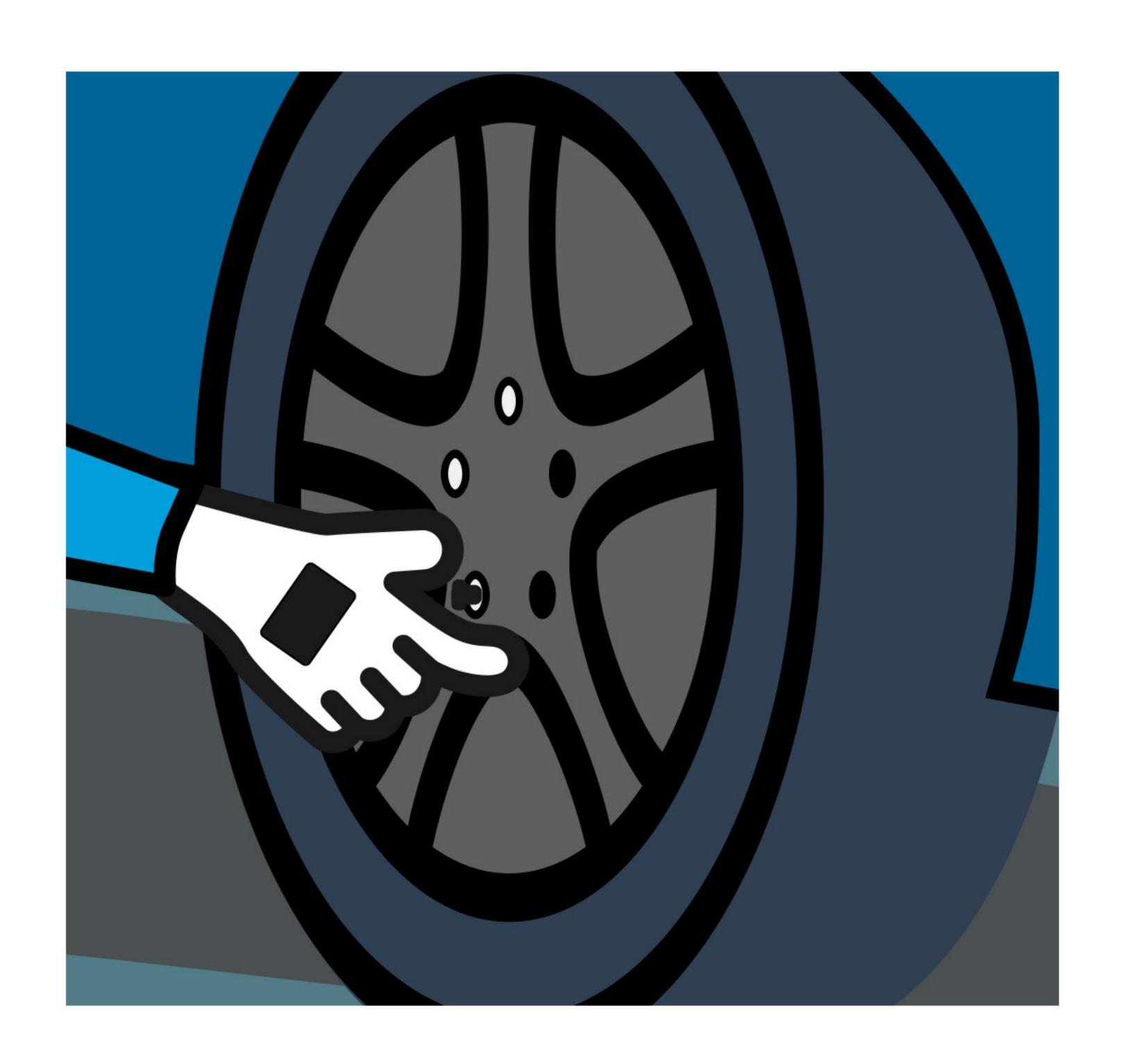
Lower car. Tighten lug nuts with wrench.
